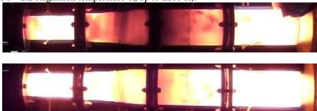
Fig 3. Durability tests of the combustion chamber made of C/SiC.
