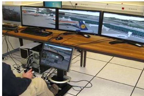
Fig. 4: PycsHEL (early stage of development) – prototyping and design bench of systems for helicopters of the future.
