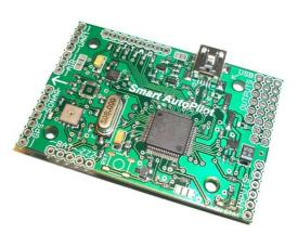
(IC) package. DMP performs calculations (angular rates integration, gyroscope drift correction, extended Kalman filtering) in order to get orientation in space in quaternion representation at the frequency of 200Hz, which significantly helps to reduce general CPU load.
