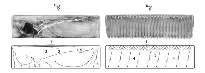
Figure 1. Flow separation on flat and wavy wing surface with similar profile:  $Re=1.5\times10^5$ , free stream turbulence level  $\epsilon$  =0.04%, angle of attack  $\alpha$ =9°, angle of sweep  $\beta$ =15°. 1– laminar boundary layer; 2 – line of separate laminar boundary layer; 3 – separation bubbles; 4 – reattached turbulent boundary layer; 5 – large scale vortexes structures; 6 – reverse flow.
