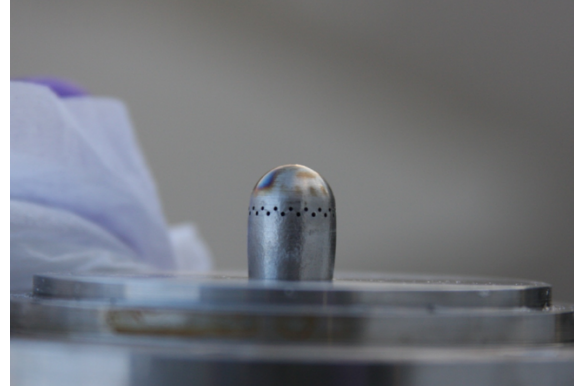
(b) Damage to Hastelloy X pintle after hot-fire 6
