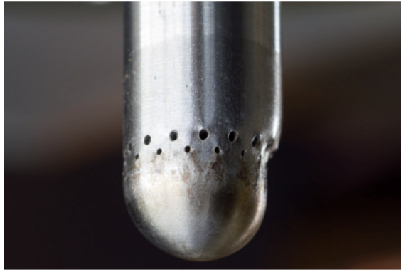
(a) Damage to 304SS pintle after hot-fire 4
