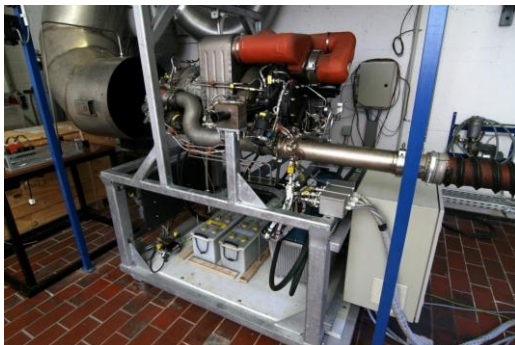
Figure 1: APU GTCP 36-300 on test rig
