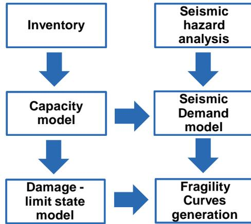
Figure 1: Derivation process of analytical fragility curves.
