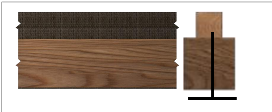
Fig.12-b. Ardwood application on a beam, lateral view and section. Connection between Ardwood element and beam is made with Ardfix connectors. The intrados of the beam is reinforced with a carbon fibre lamina or a fabric.
