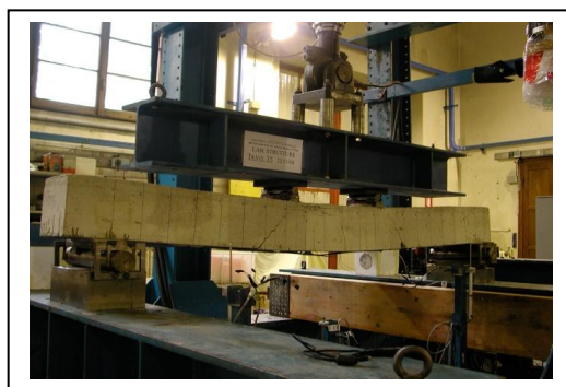
Fig.8a. Four point Flexion test on a concrete beam reinforced with n°3 layer of 300g/m 2 of high modulus (E=390 GPa) carbon fibre. No delamination has been detected during test.
