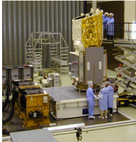
Figure 1: Aeolus Structural Model (STM) on the ESA/ESTEC Multishaker being prepared for vibration testing (source: ESA/Estec)
