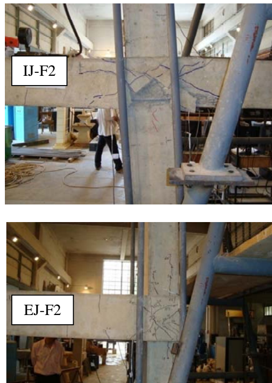
Figure 4: Failure mode of the joint specimens
