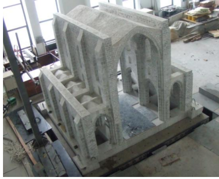
Fig. 6. Fossanova physical model (UPM) in scale 1:5.5 tested on shaking table.
