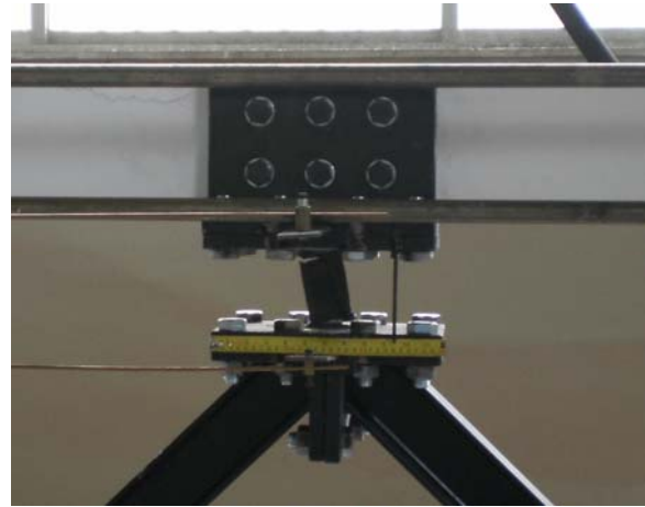
Figure 18: Failure mode of the link element (F2)
