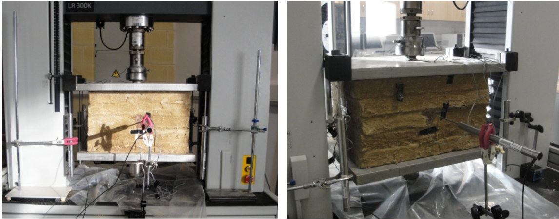
Figure 1: Pictures of the experimental setup used in the implementation of compressive loading-unloading tests on an adobe masonry assemblage composed of five full-size adobe bricks and earth mortar joints.
