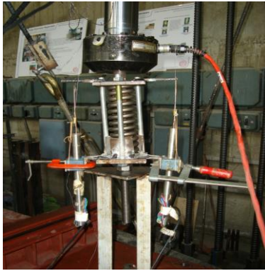
Figure 4. Test for measuring the spring stiffness
