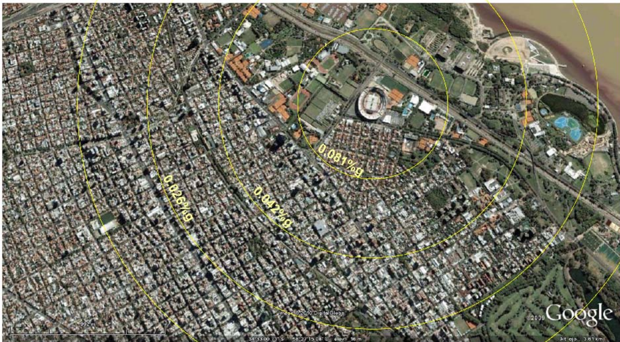
Fig. 7. RMS horizontal acceleration on soil at 500, 1000 y 1500 m from River Plate stadium
