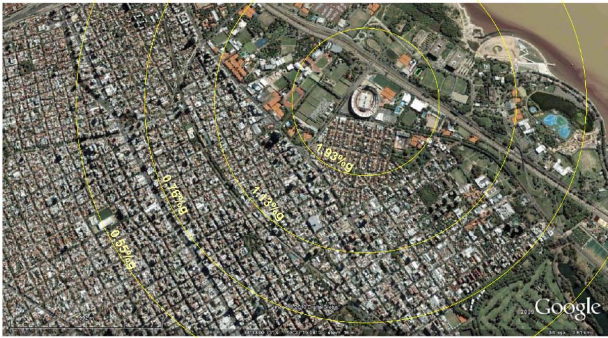
Fig. 10. RMS building top accelerations for buildings with 2 Hz of natural frequency computed at 500, 1000, 1500 and 2000 m distance from the River Plate stadium
