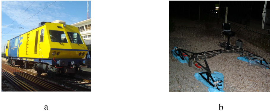
Figure 13 – Equipments for measuring the track unevenness: a) recording car; b) device for measuring the rail corrugation.
