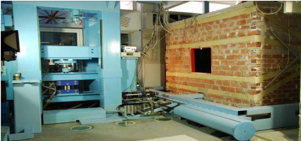
Figure 4: The reaction-actuating unit of the shake table facility (left) with a masonry structure (right).
