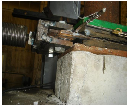
Figure 7d. Failing mode of the unit slice specimen with the presence of the compressive stress field.
