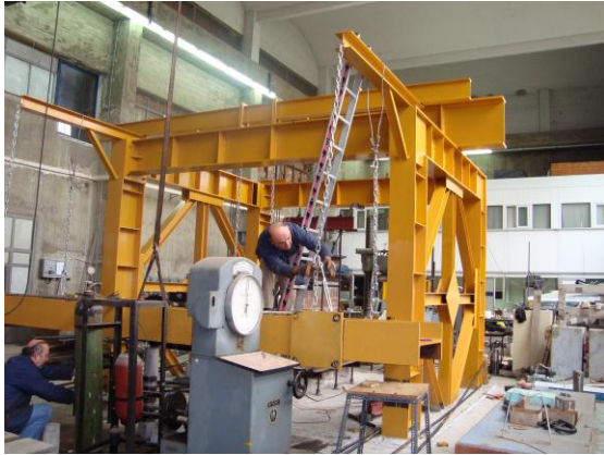
Figure 11a. The strong reaction frame of Aristotle University.
