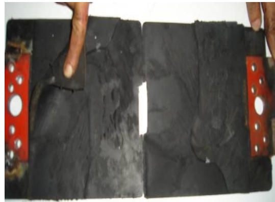
Figure 7b. The debonding of the elastomer from the steel plating at the end of this loading sequence.
