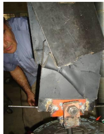
Figure 6b. Failing mode of the unit slice specimen without the presence of the compressive stress field.
