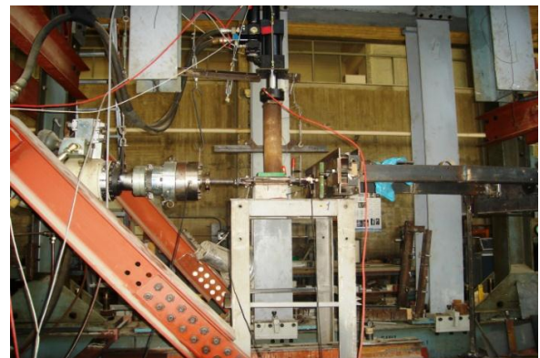
Figure 3b. Loading arrangement of a unit slice with the simultaneous application of a compressive stress field.
