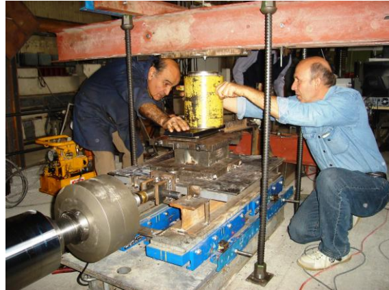
Figure 11b. The 250mm x 200mm elastomeric bearing at the strong reaction frame
