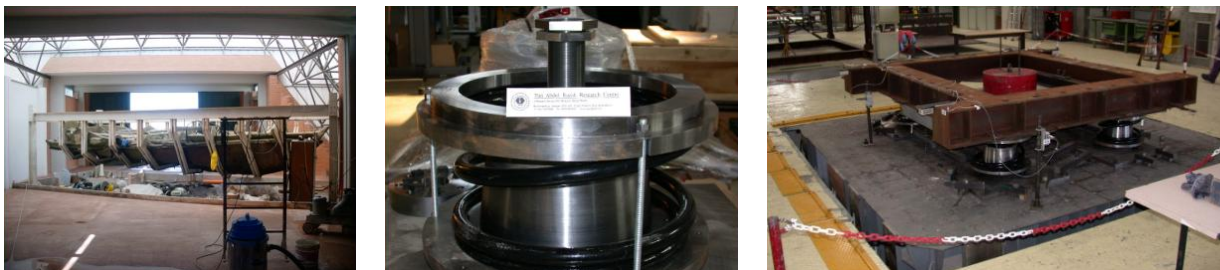
Figure 33: Roman ship excavated near Ercolano (Naples) and exhibited in the local museum, which is located in seismic zone 2 (left); one of the four 3D isolators manufactured to protect it (at the centre); shake table tests of its SI system (right).
