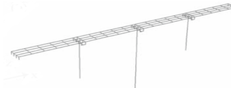
Figure 3: Overview of the fixed base, 1D superstructure finite element model (1D-Fixed).
