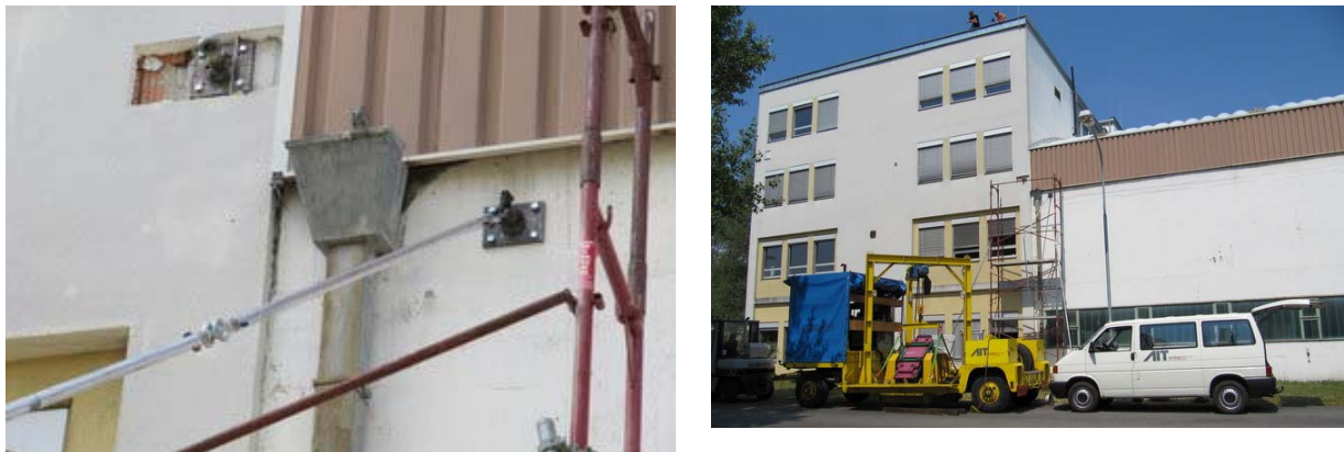
Figure 4 left: connection with the building; right: position of the exciter mass
