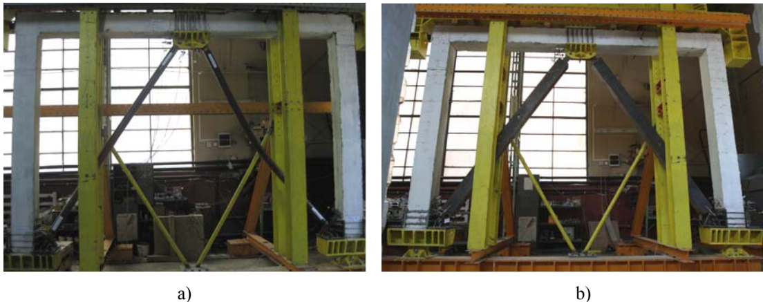
Figure 11: Photos after the test with frame strengthened with CBS a) and strengthened with BRB b)
