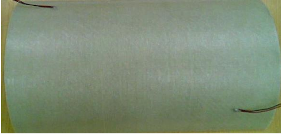
Figure 10: Configuration of the cylindrical panel with the sensor and actuator – the actuator is located above delaminated area 5 [cm] from the upper panel edge and the sensor 5 [cm] from lower panel edge.
