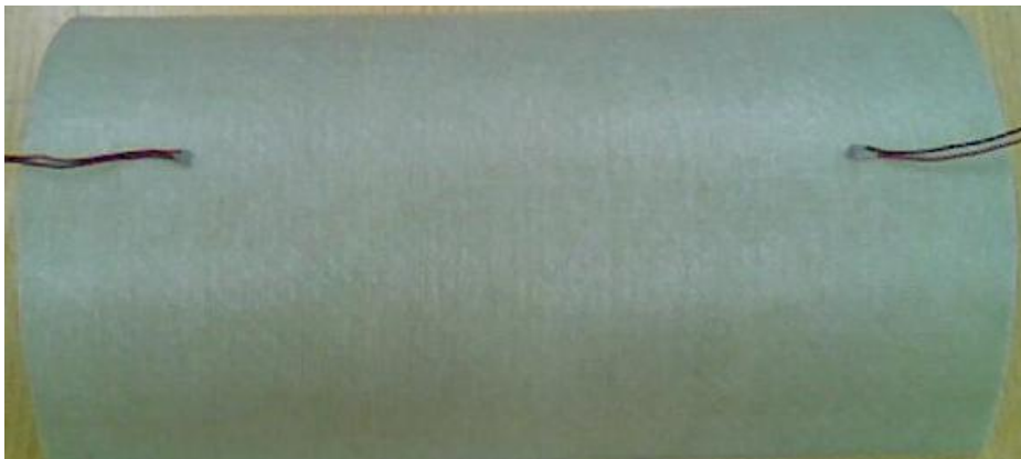
Figure 6: General configuration of the cylindrical panel with one sensor and one actuator – they are located parallel to the delaminated area.
