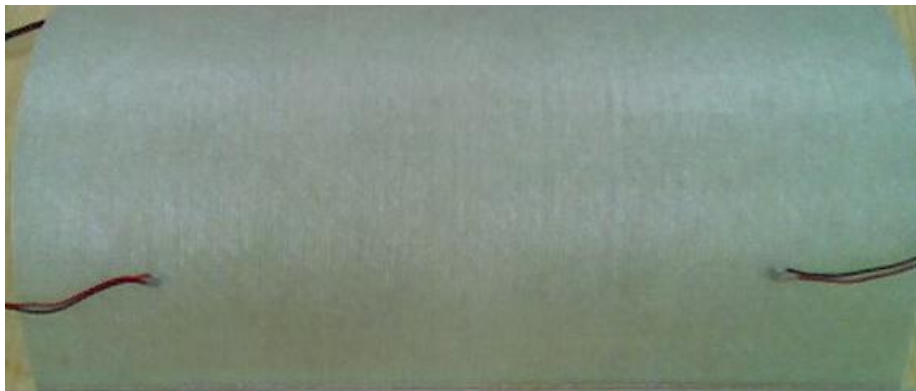
Figure 8: Configuration of the cylindrical panel with the sensor and actuator – they are located below delaminated area 5 [cm] from the panel edge.
