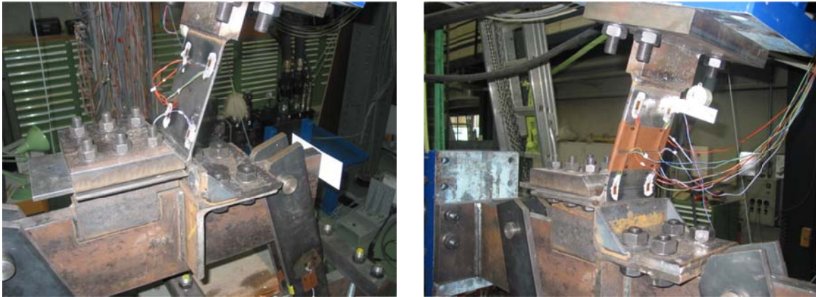
Figure 2: Specimens being tested; left, view from “inside” of tank; right, view from “below” the tank’s base plate.
