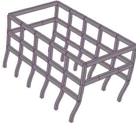
Figure 9: Deformed shapes of the fundamental vibration modes for one principal directions.
