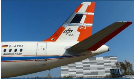
AFLoNext flight test with HLFC installation on the fin of Airbus A320 (Courtesy: DLR)
