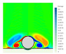
**Figure 1**: Damage caused by a single particle impact.
