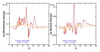
Figure 1: Ux and Uy velocity at line y=-4: (Left) high order and low order solvers and (right) high order and ROM with 3 and 5 retained modes.
