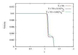
The calculated velocity field in an elastic-plastic piston problem with aluminum using the DG method with quadratic polynomials and different hardening models.
