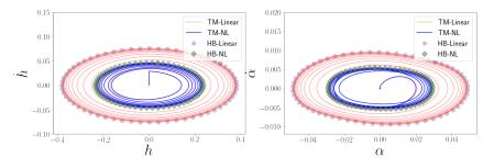
Figure 1: Position-velocity diagram for an aerofoil LCO at  $M_{\infty} = 0.8$  with linear and nonlinear structure
