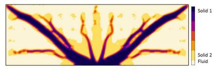
Figure 1 Optimised two-material convectively cooled heat sink design
