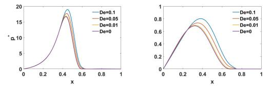
Figure 1: Non-dimensional pressure  $p^* = \frac{p}{\mu U L/h_{max}}$  (where  $h_{max}$  is the maximum of the film thickness), for a parabolic slider with minimum film thickness (left)  $h_{min}=0.1$  and (right)  $h_{min}=0.5$ . The lubricant cavitates where  $p^*=0$ .
