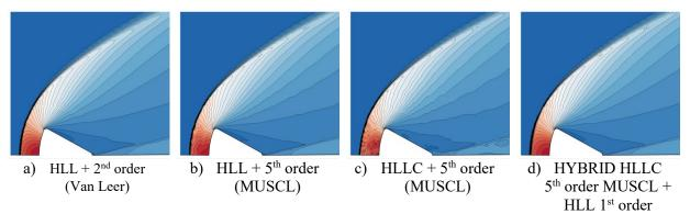
Figure 1: Steady 2D inviscid flow at Mach 32.4 around the Apollo 4 re-entry capsule.
