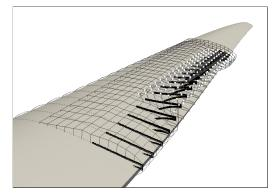
Figure 1: FFD box moving trailing edge (black) into flap position. Only a select few control points (white) are moved, creating a smooth flap-transition along the blade.
