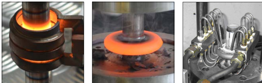
Figure 1: Integrated thermomechanical forming process, cf. [20]
