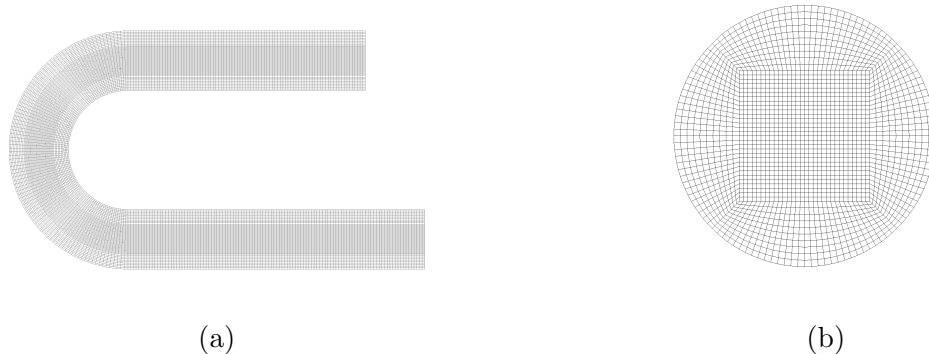
Figure 2: View of the reference mesh containing 630,000 cells. (a) Midplane (b) Cross-section of the tube
