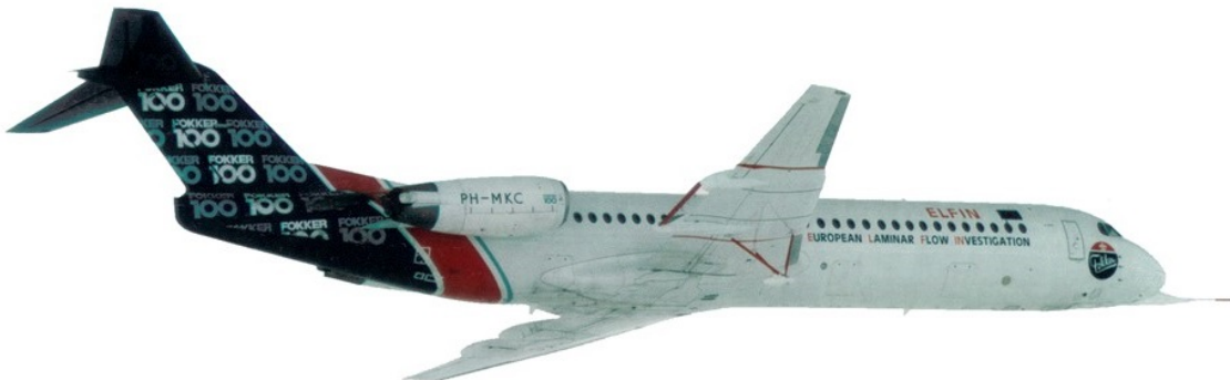
Figure 1: Fokker F100 with laminar flow glove on starboard wing
