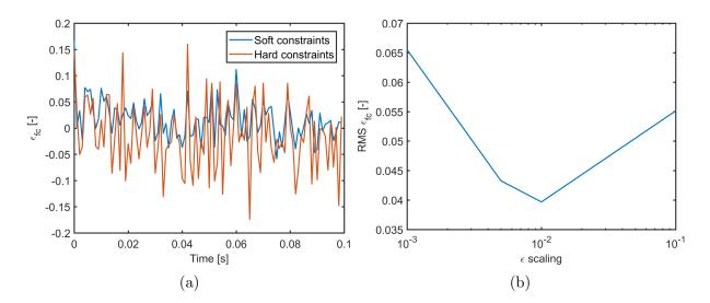
Figure 3: Relative error on total vertical contact force (a) and RMS relative error on total vertical force (b) for different scalings of the penalty factor  $\epsilon$
