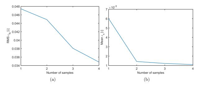
Figure 2: RMS relative error on total vertical contact force (a) and mean global relative error on displacements (b) for different amounts of MCMEM samples
