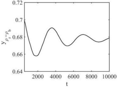
Figure 1: Maximum height of the contour evolution with the number of time steps for  $\sigma = 5 \cdot 10^{-3}$ . The contour is located where the heavy fluid density (red: $\rho_r$ ) is equal to the light fluid density (blue: $\rho_b$ ).
