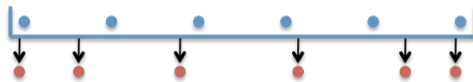
Figure 6: Providing equidistant coupling points (blue) for the interpolation but requesting point values for non-equidistant points (red) for preCICE
