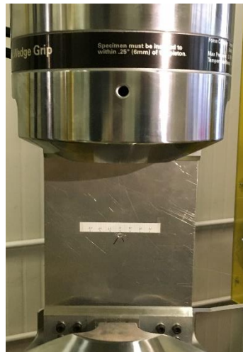
Figure 3: Detail of the specimen mounted on the MTS Landmark machine; an artificial notch can be noted in the middle of the plate
