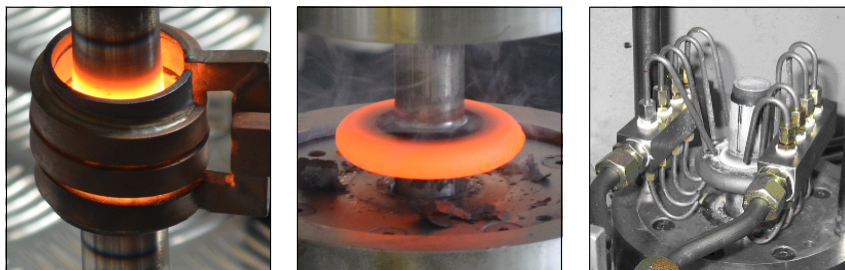
Figure 1: Integrated thermomechanical forming process, cf. [19]
