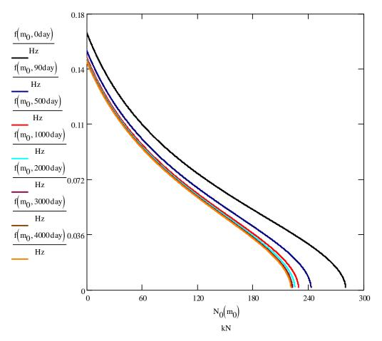
Figure 4. Critical buckling load over time
