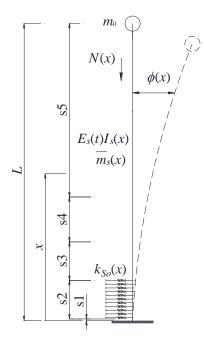
Figure 3. Frame element model in free vibration
