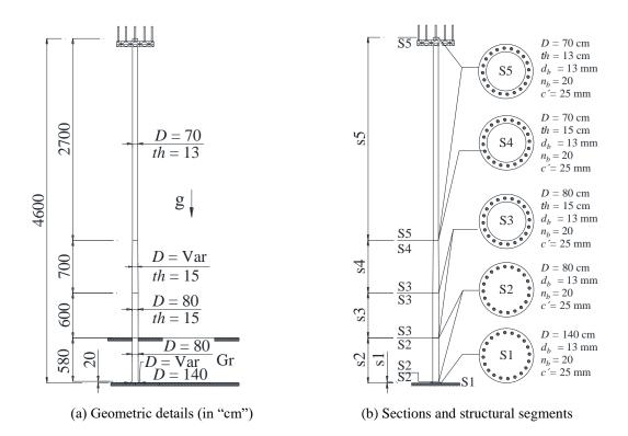
Figure 2. Subject reinforced concrete pipe
