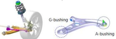
Figure 1. G bushing position of lower arm in the MacPherson suspension
