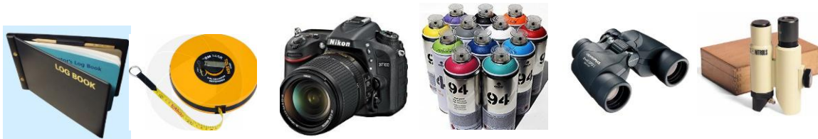
Figure 2: Typical inspection equipment required to conduct visual inspection
