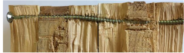
Figure 5 Metal dowel shear test
