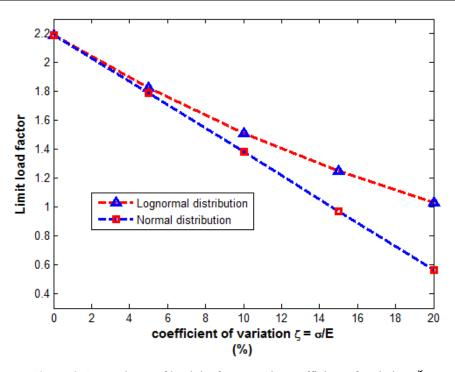
**Figure 3**: Dependence of load the factor on the coefficient of variation  $\xi$
