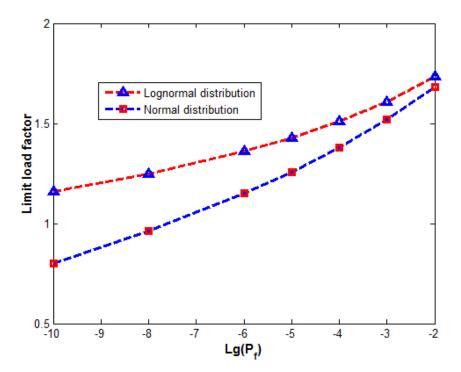
Figure 4: Dependence of the load factor on the failure probability
