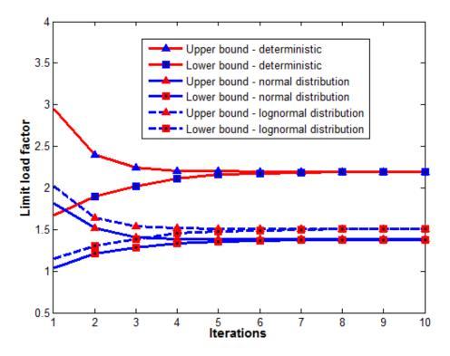
Figure 2: Convergence of the limit load factor in case of deterministic and random strength.
