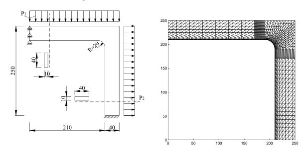
Figure 7: The geometrical dimensions and FE-mesh
