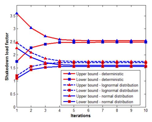
Figure 9: Shakedown load factor with random strength, deterministic loads.
