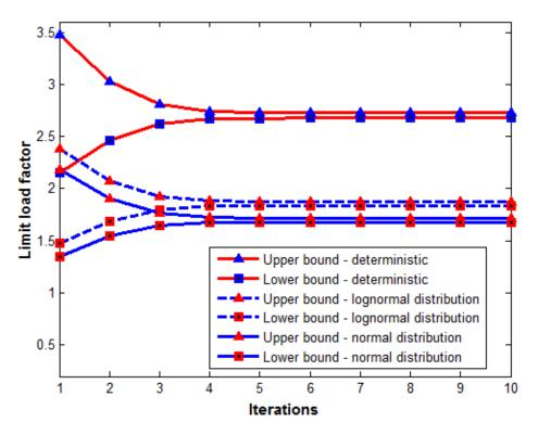
Figure 8: Limit load factor with random strength, deterministic loads.
