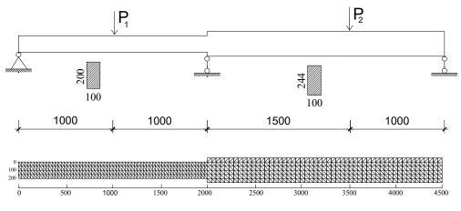
Figure 1: Two-span beam and FE mesh with T3 elements
