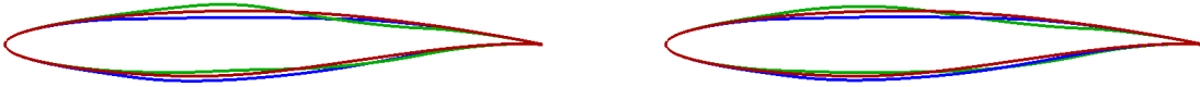
Figure 5: Comparison of the initial (red curve), \mu_F optimal (blue curve) and \sigma_F optimal (green curve) geometries designed by the pFOSM (left) and the iPCE (right).
