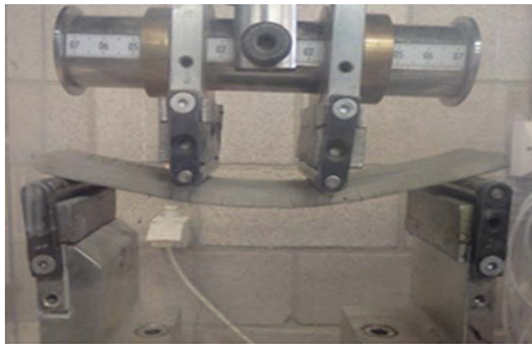
Figure 1: 4-point bending tests arrangement
