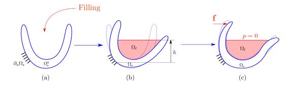
**Figure 4**: (a) Reference configuration without fluid; (b) current configuration for a given fluid height; (c) linearized vibration around a prestressed state under a small amplitude excitation **f**.
