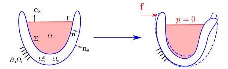
**Figure 2**: Hydroleastic problem description without pre-stress effect under a small amplitude harmonic load  $\mathbf{f}$ , with no gravity effect such that the pressure fluctuation is fixed as p = 0 on the free surface  $\Gamma$ .
