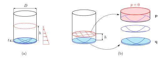
Figure 5: (a) Filling of a cylinder of diameter D=357 mm with water  $\rho_{\rm f}=1000$  kg.m<sup>-1</sup>, rigid walls and an elastic bottom of thickness t=0.357 mm made of plexiglas. The material parameters are the Young Modulus E=5.47e9 Pa and a Poisson Ration of 0.38 and the plexiglas density  $\rho_{\rm s}=1.38$  kg.m<sup>-3</sup>. The fluid height value is such that  $h\in[0,250]$  mm; (b) Hydroelastic vibrations around the pre-stressed state for a given fluid height h.
