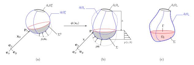
**Figure 1:** (a) Reference configuration of the internal surface of a tank; (b) Current configuration of internal surface of a tank loaded by hydrostatic follower forces; (c) Linearized hydroelastic vibration around a pre-stressed state without gravity effects
